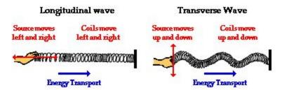
In **longitudinal** waves, the particles move parallel to the direction the wave travels. A sound wave traveling through air is a longitudinal wave.
